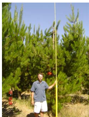
Photo 1: The telescopic measuring pole used to measure the height of GM pine trees.
